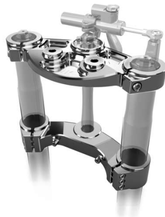
Human Design Weight: 3 kg Safety factor: 2.7 Cost: $
