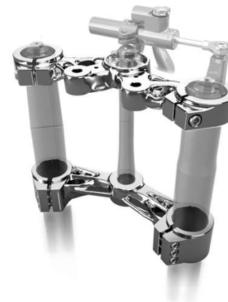
3 Axis Generative Weight: 2.3 kg (-23%) Safety factor: 2.3 Cost: $
